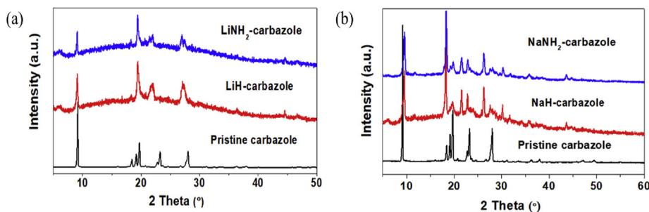
Fig. 3 – XRD patterns of (a) lithium carbazolid and (b) sodium carbazolid using different metal-based compounds as metal precursors.
