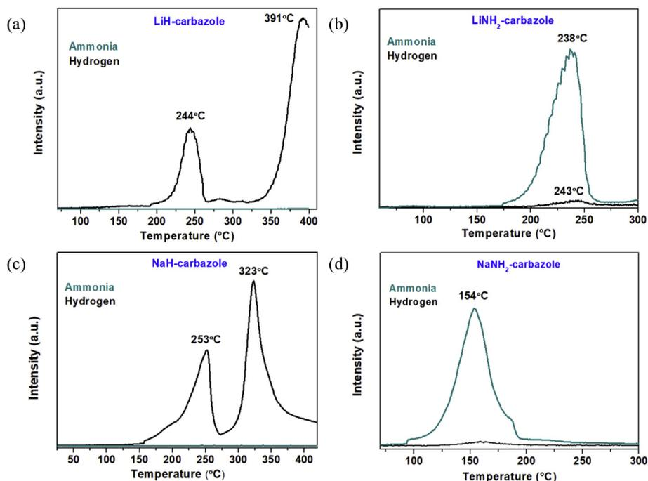
**Fig. 1** – TPD-MS of the syntheses of metallo-carbazolides using (a) lithium hydride, (b) lithium amide, (c) sodium hydride and (d) sodium amide.
