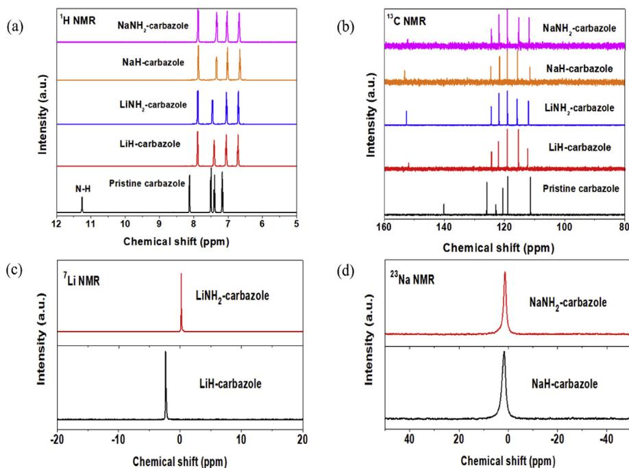
Fig. 4 – (a)  $^1\text{H}$  and (b)  $^{13}\text{C}$  NMR of metallo-carbazolides as compared to pristine carbazole in  $\text{DMSO-d}_6$ . (c)  $^7\text{Li}$  and (d)  $^{23}\text{Na}$  NMR of lithium and sodium carbazolid, respectively.
