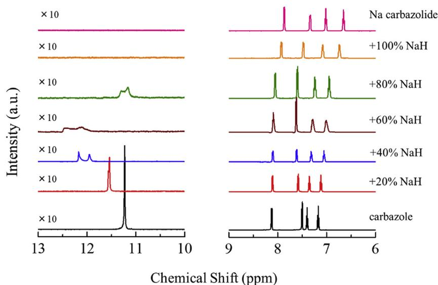
**Fig. 5 – Quasi in situ  $^1\text{H}$  NMR of sodium carbazolidide by gradually increasing the percentage of using sodium hydride as compared to pristine carbazole in  $\text{DMSO-}d_6$ .**
