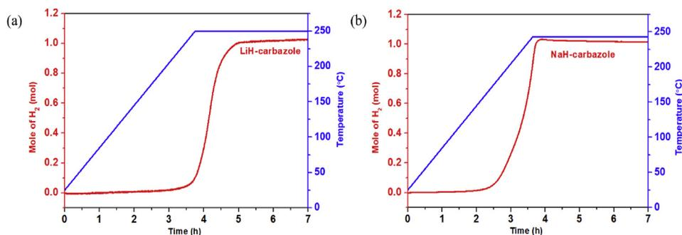
**Fig. 2** – Hydrogen release upon the heat treatment of ball milled (a) LiH-carbazole and (b) NaH-carbazole at 250 °C and 243 °C, respectively.
