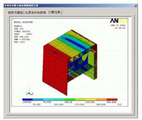
Fig.3 Equivalent stress distribution by FEM
