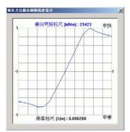
Fig.5 Bending moment and curvature relationship by SM
