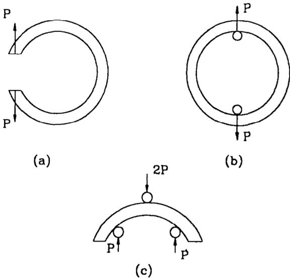
Figure 5 Ring or curved beam specimens<sup>14</sup>
