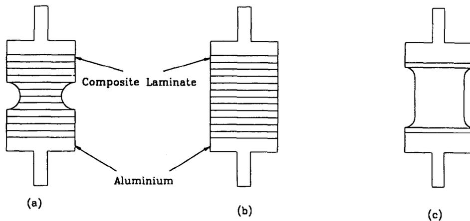
Figure 2 Variations of flatwise tension test specimen<sup>3,7-10</sup>
