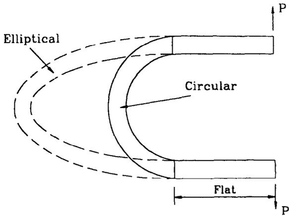
Figure 4 Semicircular or elliptical specimen<sup>13</sup>
