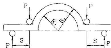
Figure 8 Four-point curved beam specimen
