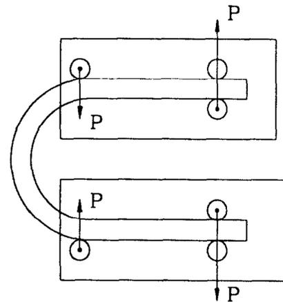
Figure 7 Pure moment on curved beam<sup>12</sup>
