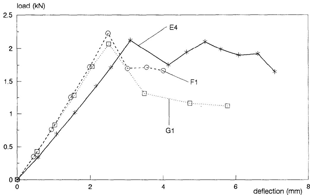
Figure 13 Typical load-deflection curves of the four-point curved beam
