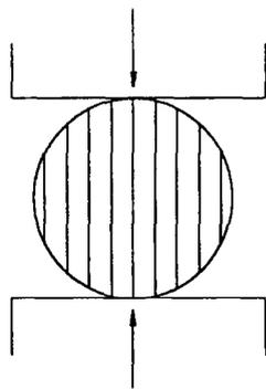
Figure 3 Diametrical compression disk specimen<sup>11</sup>
