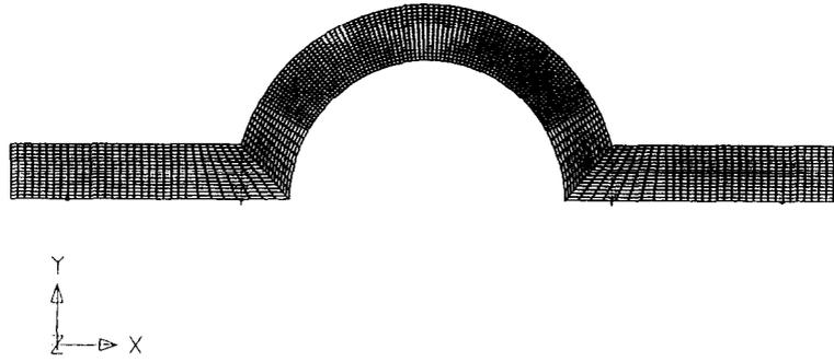
Figure 10 Curved beam finite element model
